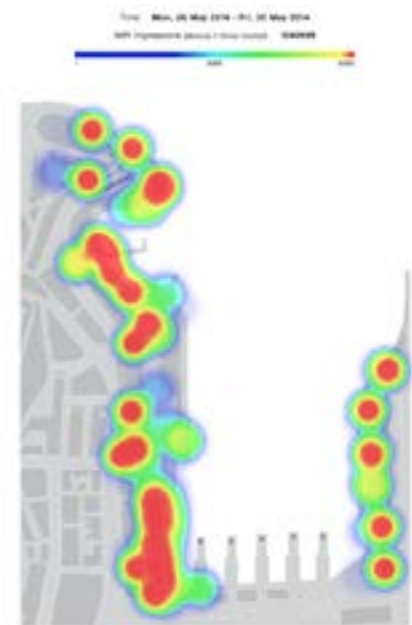
Figure 5: (Below) Ruckus cloud-hosted SPoT provided a heat map of visitors, allowing Vivid to oversee visitor density and follow their path throughout the festival.
