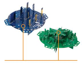
Patented smart antenna arrays integrate up to nine high-gain vertically-polarized and nine horizontally-polarized antenna elements. This enables up to 4224 potential antenna combinations, up to 9 dBi gain and up to 17 dB of interference rejection, thereby delivering unprecedented range extension and signal reliability. The dual polarized smart antenna increases the effectiveness of spatial-multiplexing, resulting in higher data rates.
